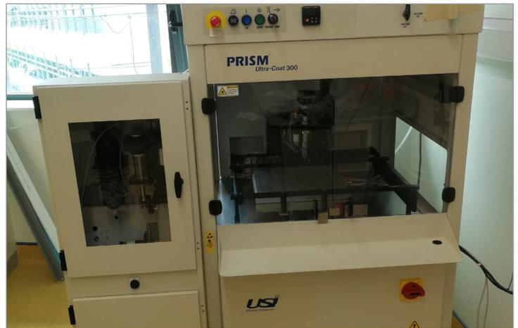
▲ Spray coater machine – one of the laboratory equipment that was contaminated
